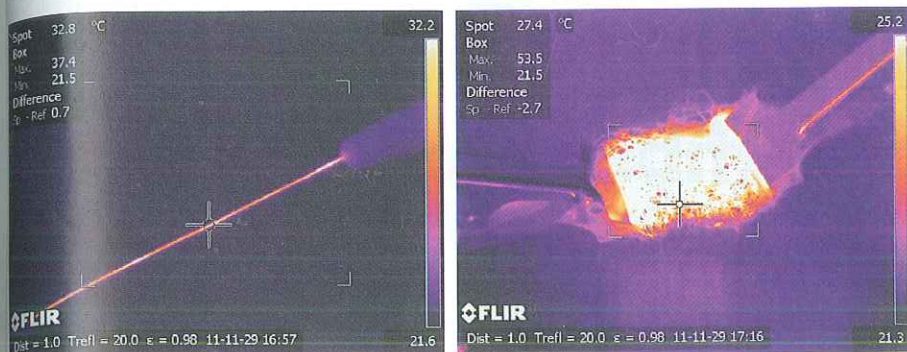
Fig. 4 Infrared camera image of single fiber (left) and nonwoven fiber mat (right)
