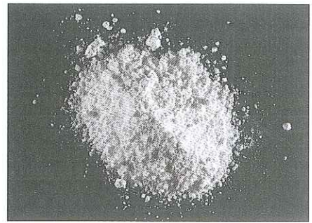
The centrifugal sifter removes agglomerated particles to leave an end product with a particle size averaging 2-5 µm.
